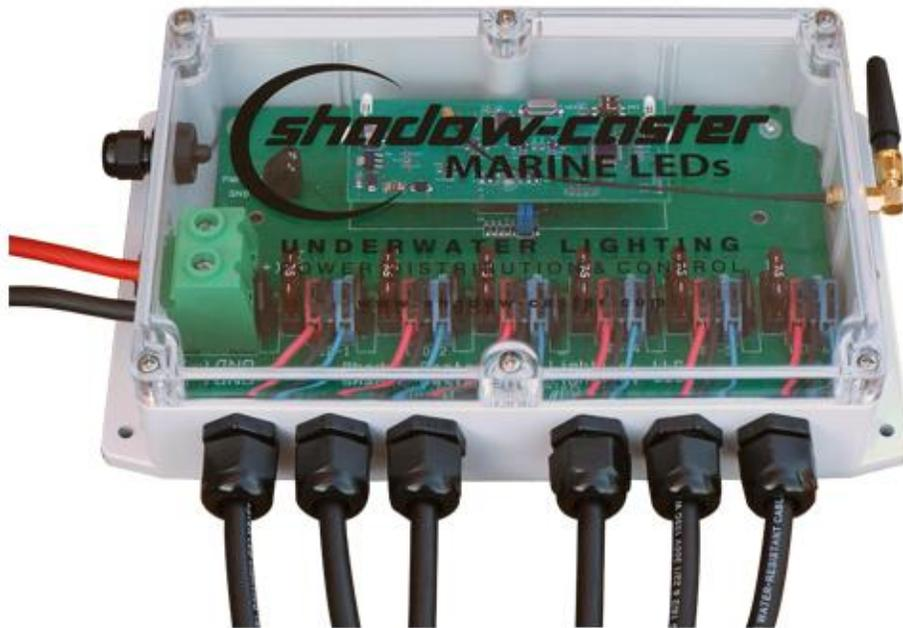
**SCM-PD shown with optional wireless Controller Installed.**
