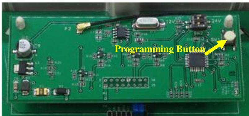
If the remote FOB must be replaced, the new one can easily be coded to the wireless receiver. To do this, power the PD Box on, then press the programming button on the receiver and release. Then press and release the MODE button on the wireless receiver, repeat this until the code is picked up by the receiver. This can be verified by seeing the Shadow-Caster Lights changing color. Note that the wireless controller will only support one remote at a time.
